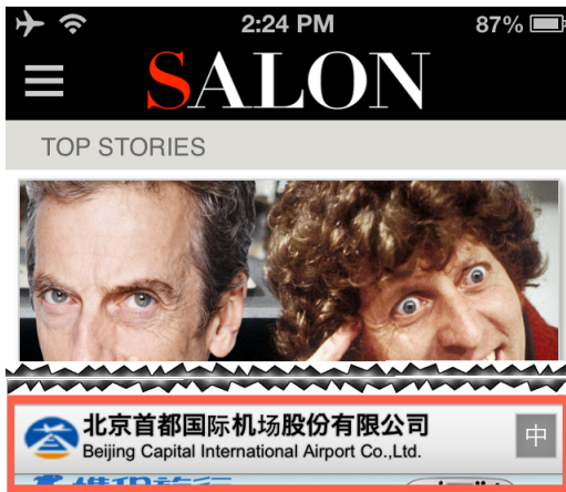
Figure 3: Screen capture of content injection by a Chinese ISP in November, 2013. The highlighted region at the bottom should be an advertisement from a US company.
